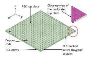
Fig. 2: The  $8\lambda \times 8\lambda$  simulation model at 28GHz with Huygens' sources arranged around the box perimeter at half wavelength apart. The equispaced brown copper rods constitute the artificial dielectric medium.
