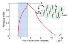
Fig. 1: Forming an effective artificial dielectric medium by arranging equispaced conductive rods. The plot relates n to spacing b at f = 28GHz and r = 0.25mm. The shaded portion has real n < 1 at  $b < \lambda_0/2$ .  $\vec{E}$ ,  $\vec{H}$  and  $\hat{k}$  are the E-field, H-field and wave propagation direction respectively. The E-field is polarized along the direction of the rods.  $\varepsilon_r$ ,  $\mu_r$  and n can be extracted using the S-parameters.
