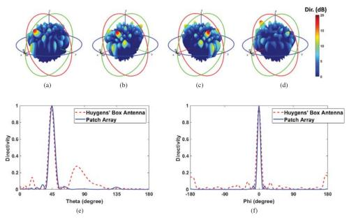
Fig. 3: Simulated radiation patterns. (a) - (d) shows radiated beams for elevation  $\theta = 45^{\circ}$  at  $\phi = 0^{\circ}$ ,  $\phi = 22.5^{\circ}$ ,  $\phi = 67.5^{\circ}$  and  $\phi = 275^{\circ}$  respectively. (e) 2D radiation patterns at  $\phi = 0^{\circ}$  plane (f) 2D radiation patterns at  $\theta = 45^{\circ}$  plane.
